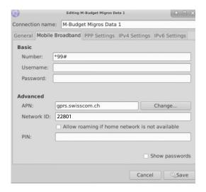
Edit now the settings for this GSM Connection and enter the data according to the following table:
