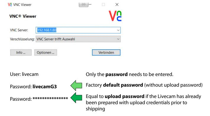
This opens a connection to the Livecam computer with Linux operating system:
