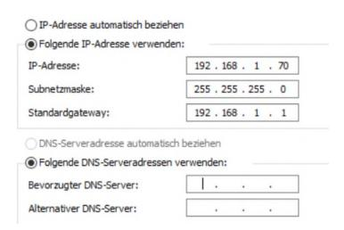
Download and install a **VNC software** to establish the connection, for example VNC Viewer. Enter the fixed IP of the camera to connect:
