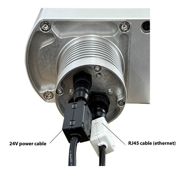
The ferrite elements are installed on the cable strands close to the camera. Installing them on the opposite side of the cable is possible but will be less beneficial for the camera.
