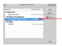
Open up the **edit connections menu** and make a left mouse-click on the mobile broadband connection and press "Edit".
