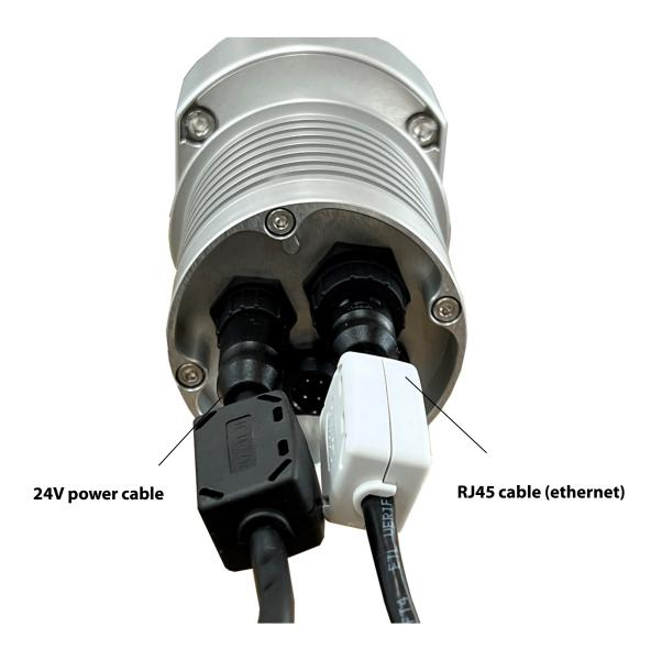
The ferrite elements are installed on the cable strands close to the camera. Installing them on the opposite side of the cable is possible but will be less beneficial for the camera.
