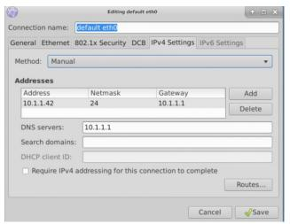
When entering the subnet mask (Netmask), the values will be indicated in binary power format, for example:
