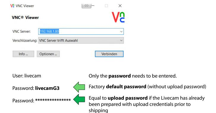
This opens a connection to the Livecam computer with Linux operating system:
